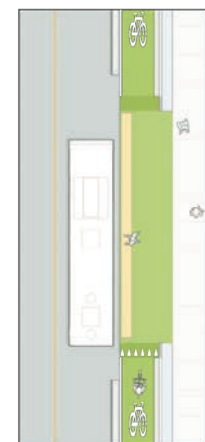
FIGURE 5.26 Raised Bike Lane at Transit Stop
