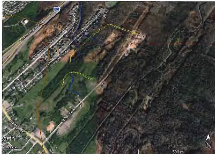
Figure 12. Possible areas between Mud Lake and Highway 125 to investigate for bermed wetlands to serve as storage for storm runoff.
