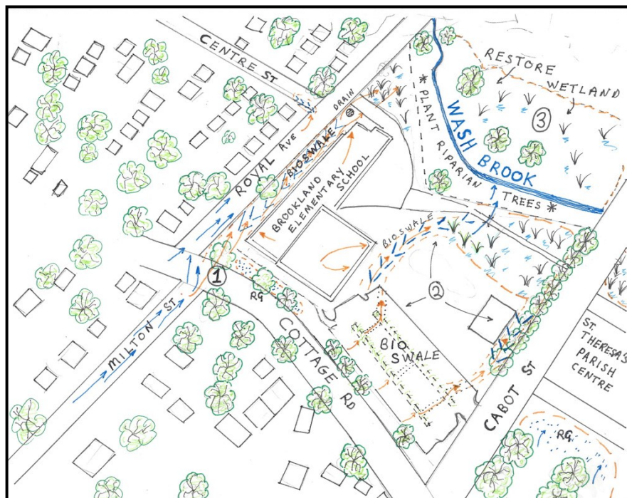
Figure 6: Brookland Elementary existing water flows (blue arrows) and possible solutions (orange arrows)
