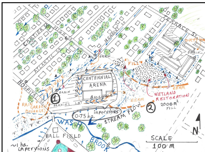
Figure 7. Floodplain zone around Centennial Arena. Blue arrows are current water flows and blue stipple is wetland. Possible bioswale installation areas are represented in blue herringbone and berms and a rain garden are suggested as orange dashed lines. Wetland areas around the arena and fill were surveyed on November 25, 2019.
