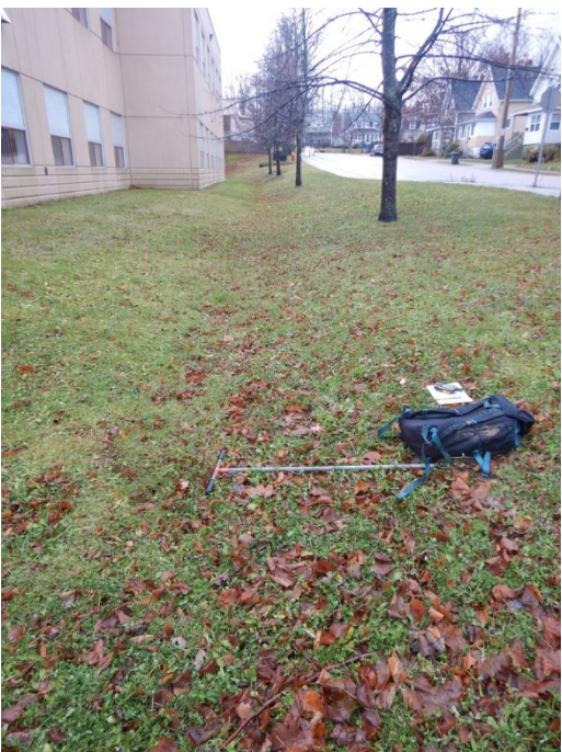
Photo 4 (at left) shows side lawn of school which will be developed to infiltrate water. Note the depression and note that at present these waters flow into a drain that is frequently plugged with leaves).
